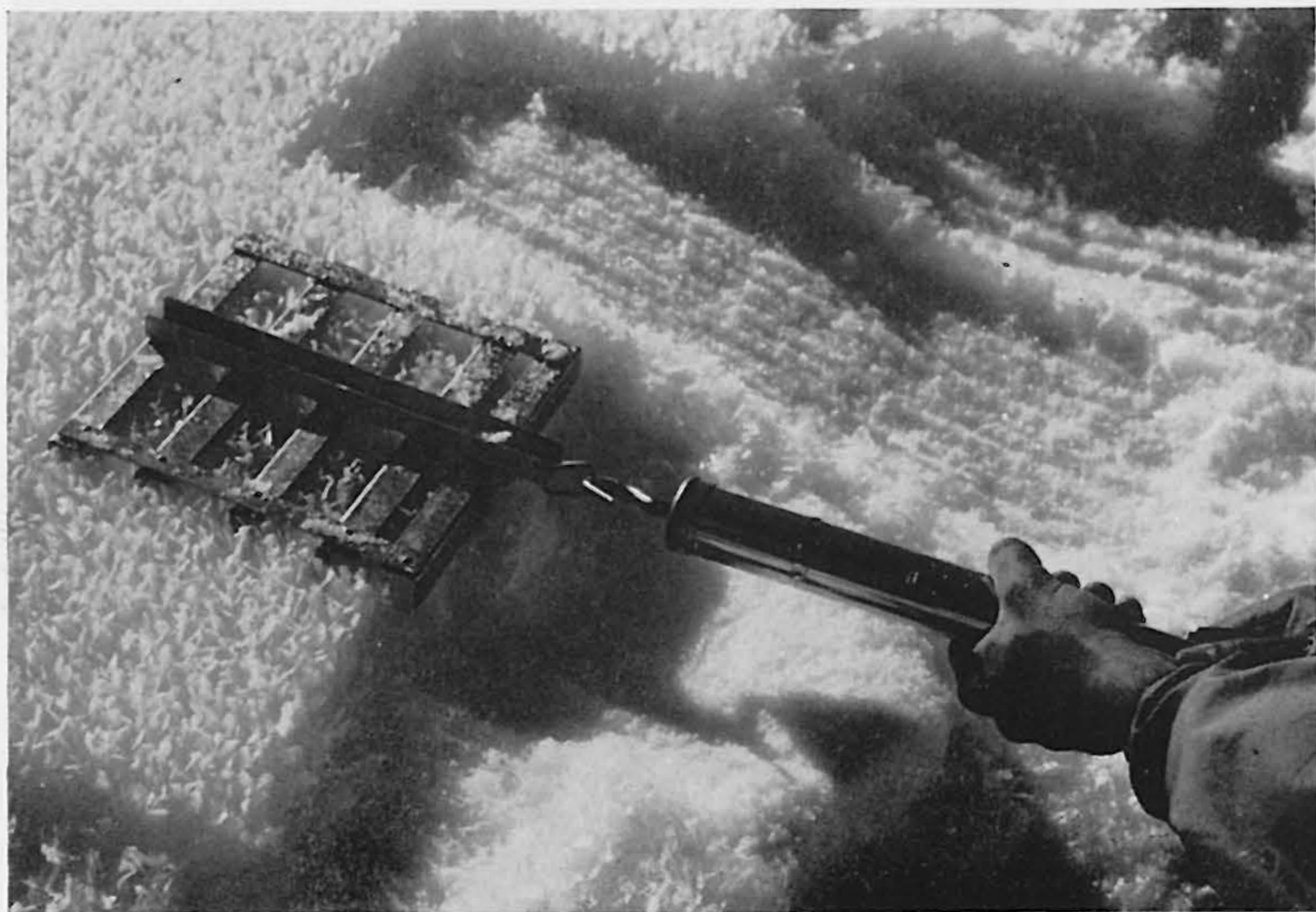
2. MEASURING THE SHEAR STRENGTH OF SURFACE HOAR IN LEAVES, WITH A FRAME OF 4 \text{ DM}^2 AND A DYNAMOMETER. THESE HOAR LEAVES WILL RESIST THE PRESSURE OF THE WEIGHT OF A NEW SNOW FALL, THOUGH THEIR SHEAR RESISTANCE IS VERY SMALL.
